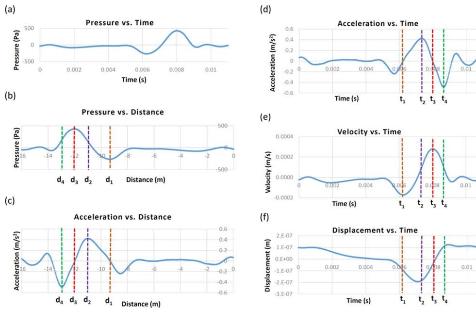
**Figure 7.** (a) Pressure as a function of time. (b) Pressure as a function of distance in front of the hydrophone. (c) Acceleration as a function of distance. (d) Particle acceleration as a function of time. (e) Particle velocity as a function of time. (f) Particle displacement as a function of time.
